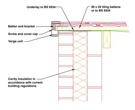
Note: When using a vapour permeable (LR) underlay, Forticrete in line with BS5250 recommend that the batten cavity is ventilated from eave to ridge
